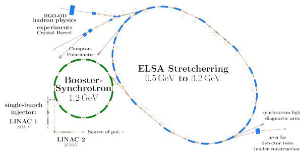
Figure 1: Sketch of the electron stretcher facility ELSA.
