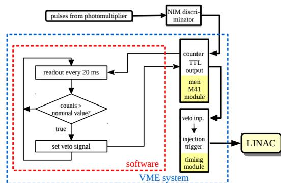
Figure 3: Scheme of the storage ring's injection control.
