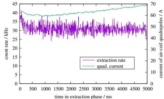
Figure 6: Electron rate (purple) and current of air-coil quadrupoles (cyan) during the extraction phase.
