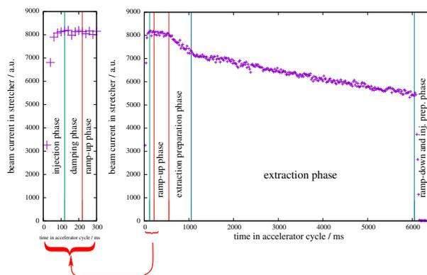
Figure 4: Photomultiplier count rate as measure of stored beam current during one accelerator cycle. On the left side the injection phase is shown in more detail.
