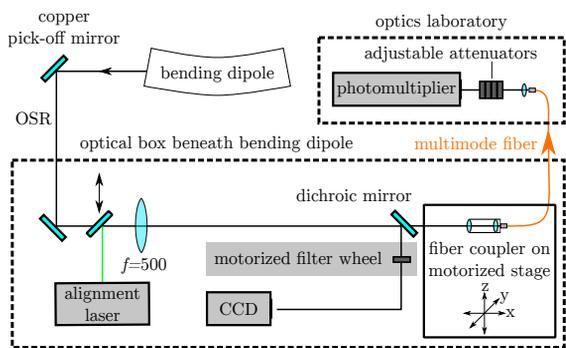
Figure 2: Layout of the M28 visible synchrotron radiation beamline with fiber connection to an optics laboratory.
