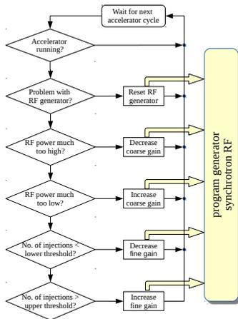
Figure 5: Control of the synchrotron RF generator.
