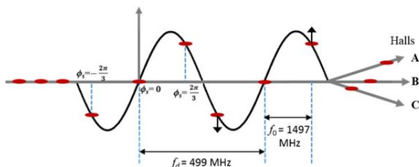
Figure 1: Bunch separation in the Jefferson Lab three-way beam spreader.
