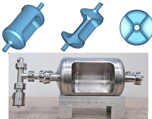
Figure 2: 499 MHz rf-dipole cavity design (top-left) with cross sections along z axis (top-center) and y axis (top-right), and the fabricated cavity (bottom).
