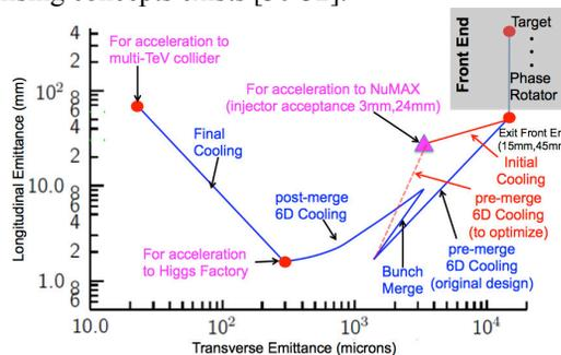
Figure 2: Transverse and longitudinal emittance evolution in a muon cooling system.
