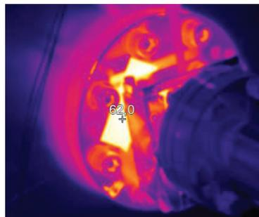
Figure 2: Infrared image of the beam pipe flange.
