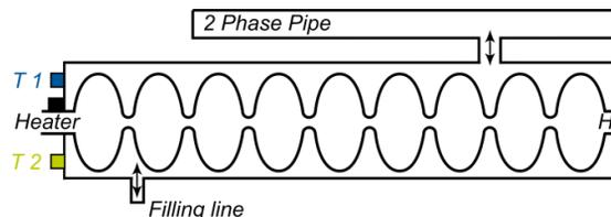
Figure 1: TESLA cavity in the LHe tank and equipped with four Cernox sensors and two heaters. The tank can be filled via the filling line and via the two phase pipe.
