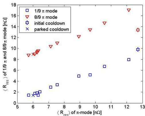
Figure 4:  $R_{res}$  obtained for the  $8/9\pi$  and  $1/9\pi$  mode as a function of  $R_{res}$  obtained for the  $\pi$  mode. Linear regression leaving out the initial cooldown results in:  $R_{8/9\pi} = 1.2 \cdot R_{\pi} + 1.8 \text{ n}\Omega$  and  $R_{1/9\pi} = 1.0 \cdot R_{\pi} - 4.7 \text{ n}\Omega$ .
