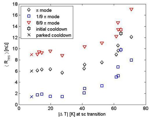
Figure 3:  $R_{res}$  measured with the three passband modes as a function of  $\Delta T$  along the cavity at the onset of sc phase transition. The lowest  $R_{res}$  was achieved in the center cells following the cycle 1 and the parked cooldown (1.4 n $\Omega \cong Q_0 > 10^{11}$  at 1.5 K).
