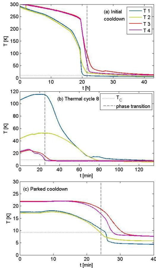
Figure 2: Temperatures measured during initial cooldown (a), a thermal cycle (b) and parked cooldown (c). The dotted line indicates  $T_c$  (9.2 K). The dashed line indicates the time when the first sensor dropped below  $T_c$ .
