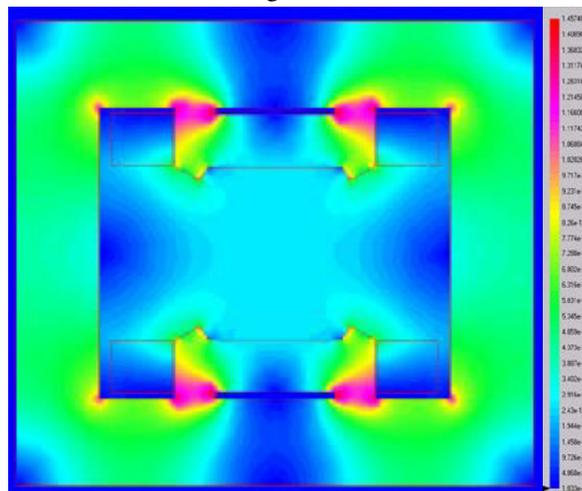
Figure 2: Magnetic field in Tesla. Each Rose shim is a triangle with base 20 mm in horizontal plane and height 8 mm at a point  $\frac{3}{4}$  along the base. Each Purcell filter is an absence of C1010 material, centred at the pole base, 4 mm in height by 72 mm in width.
