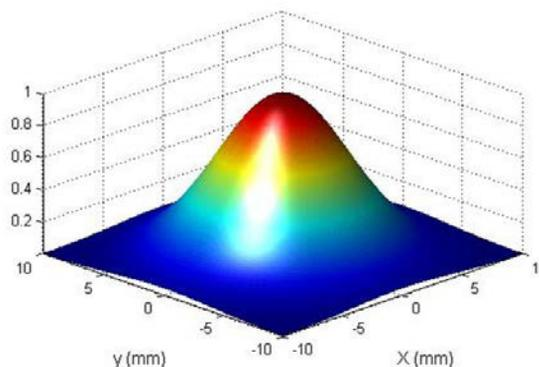
Figure 9: Gaussian distribution 325 keV, Ar+ beam.
