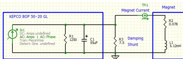
Figure 7: Damping circuit with resistances in  $\Omega$ .
