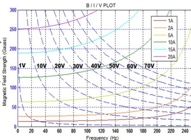
Figure 5: Magnetic field as a function of frequency for power supply sinusoidal peak current values up to  $\pm 20$  Amps and, for the case of the KEPSCO BOP 50-20 GL power supply, a maximum of  $\pm 50$  Volts.
