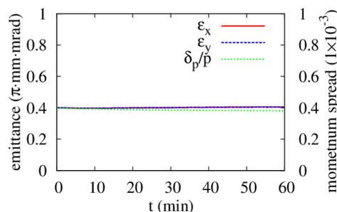
Figure 4: Cooling of 100 GeV proton beam by a bunched electron beam in the MEIC collider ring.
