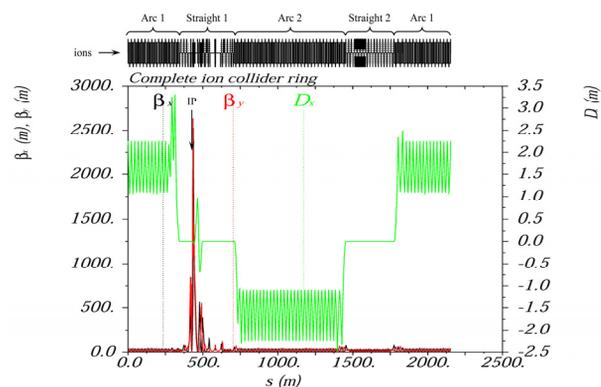
Figure 6: Complete ion collider ring optics.
