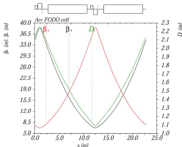
Figure 2: Ion arc FODO optics.
