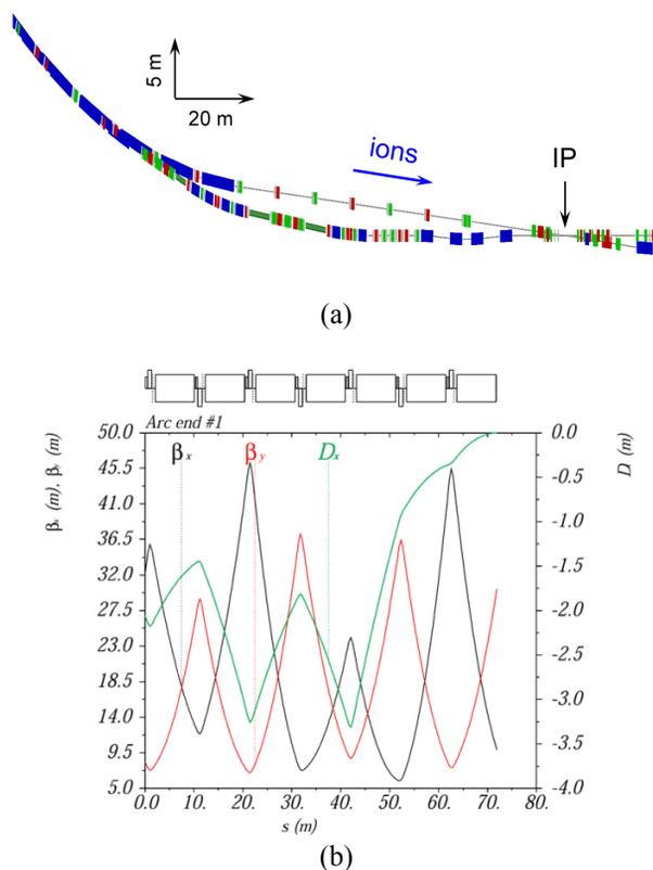
Figure 3: Geometry (a) and optics (b) of the arc end upstream of the IP.
