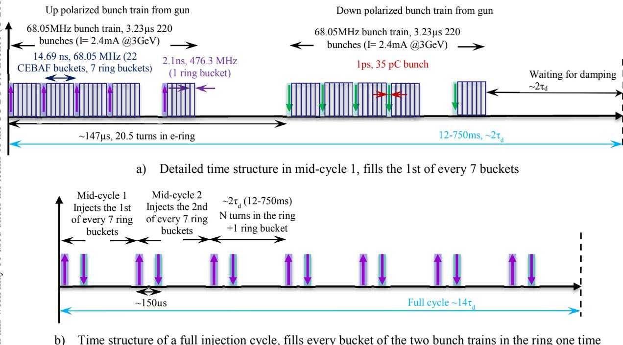
Figure 5: Injection cycles (not to scale)
