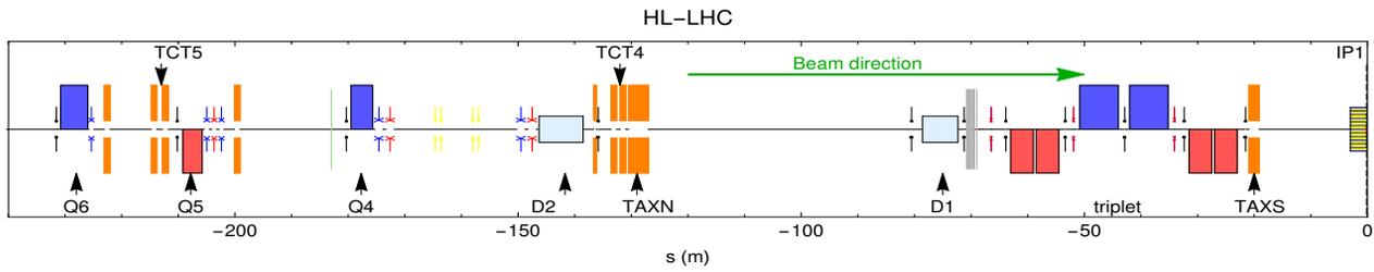
Figure 1: Planned HL-LHC layout [5] for the incoming beam in the experimental insertion region of ATLAS (IP1) with tertiary collimator pairs (TCT4s and TCT5s) highlighted above the beamline. Layout in IR5 is identical.
