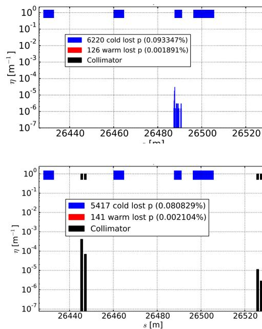
Figure 3: Loss maps in the Q5 and Q4 upstream IP5 with reduced apertures ( $8.7\sigma$ ) and without (top) and with (bottom) the installation of the TCT5 and TCT4 at  $8.3\sigma$ . The losses in Q4 are fully absorbed when TCT5 is included.
