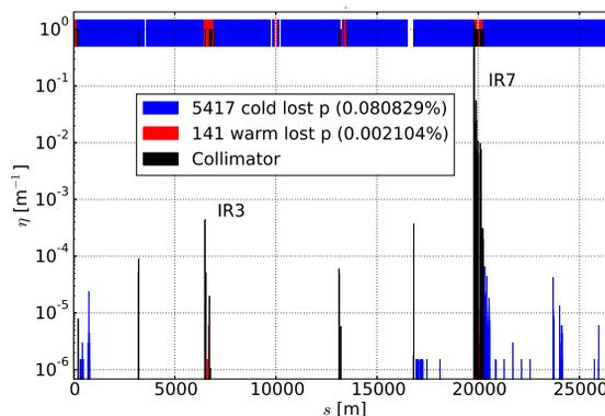
Figure 1: Example of a loss map representing the losses along the ring for Beam1 considering nominal apertures and Tertiary collimators in their nominal setting ( $8.3\sigma$ ). Black lines represent losses in collimators, blue lines losses in cold regions and red lines are losses in warm regions.
