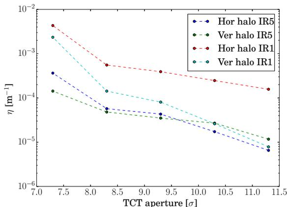
Figure 4: TCT inefficiency in IR1 and IR5 as a function of the collimator gap for horizontal and vertical halo.
