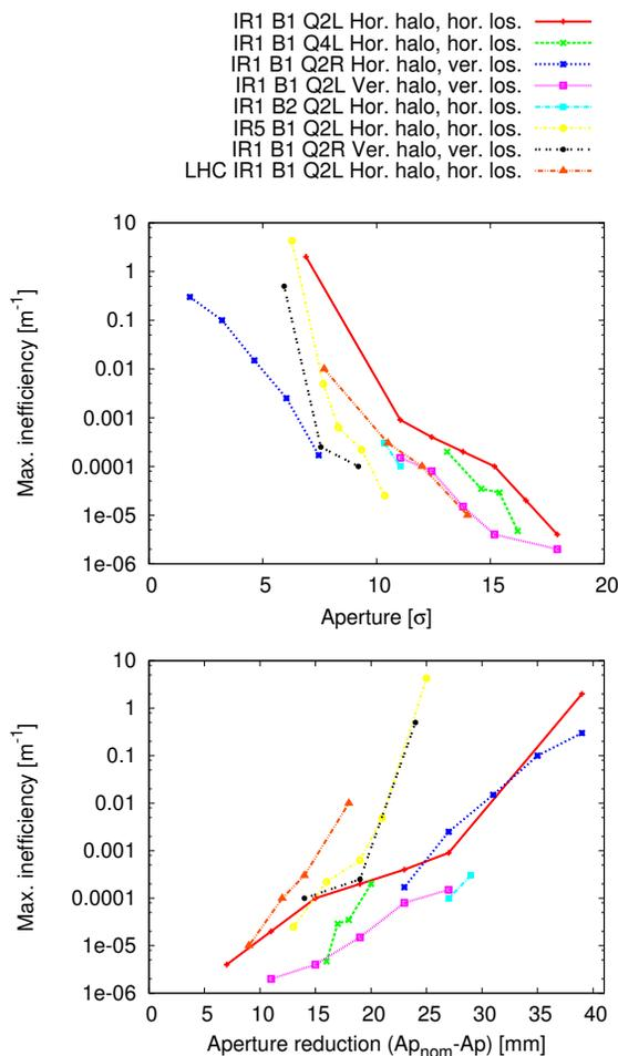
Figure 2: Maximum inefficiency  $\eta$  for different magnets and different halos and beams for aperture in beam size units (top) and as a function of the aperture reduction in millimeters (bottom) and TCT fully open.
