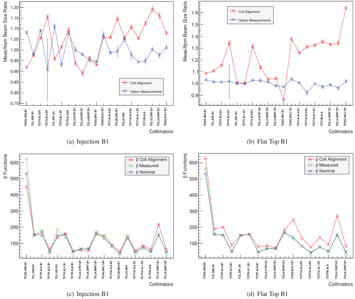
Figure 2: Beam size ratios and \beta -functions at injection and flat top for H and V collimators (except IR3).
