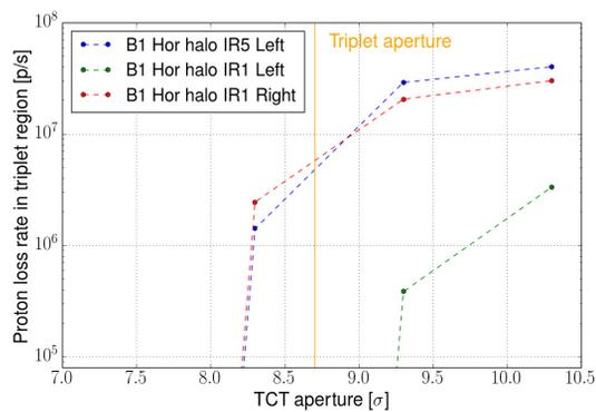
Figure 3: Integrated cleaning losses in the triplets, simulated with SixTrack, as a function of the TCT setting for HL-LHC with nominal collimator settings. The triplet apertures were simultaneously reduced to  $8.7\sigma$  and no losses were observed right of IR5. The LHC design quench limit, which now is known to be pessimistic, is at  $5.4 \times 10^6$  p/s.
