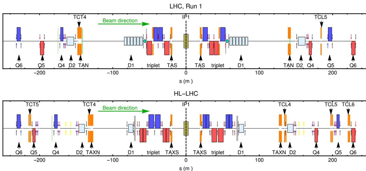
Figure 1: Layout of IR1, around the ATLAS experiment at  $s = 0$ , in the LHC during its first run 2010–2013 (top) and in HL-LHC (bottom) for B1, going from left to right. Collimators and fixed absorbers are indicated by orange color.
