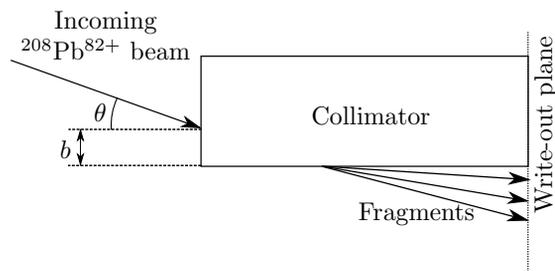
Figure 1: Schematic illustration of the fragmentation simulation. The collimator is modeled as a block of carbon. A beam of  $^{208}\text{Pb}^{82+}$  ions hits the material at an angle  $\theta$  with an impact parameter  $b$ . At the end of the collimator, the coordinates and species of all ions are written out.
