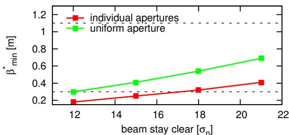
Figure 4:  $\beta^*$  reach with a coil aperture field of 11 T. The dotted lines indicate baseline and “ultimate” value. Note that the shown values present a lower limit for the given input since dispersive effects, magnet misalignments and manufacturing tolerances are not yet taken into account. There is a comfortable margin to the baseline goal so reaching it should not become a problem.
