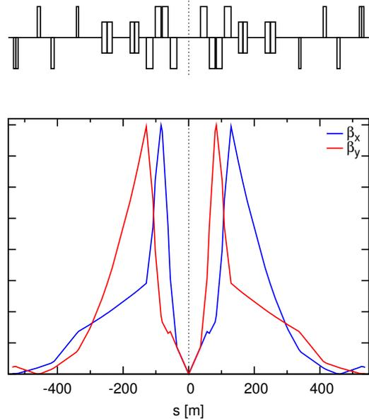
Figure 1: FCC-hh interaction region design with  $\beta^* = 0.3$  m and  $L^* = 36$  m.
