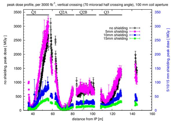
Figure 2: Radiation dose in the triplet magnets from physics debris with (right scale) and without (left scale) shielding. For 15 mm shielding and the shown integrated luminosity of  $3000 \text{fb}^{-1}$ , the dose looks acceptable [4].
