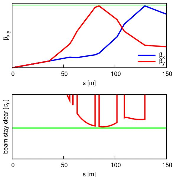
Figure 3: Principle of the  $\beta^*$  reach calculation: the triplet was rematched to have the same maximum  $\beta$  function in the vertical and horizontal plane (top). After rematching the crossing angle orbit correctors and setting the apertures, the beam stay clear was evaluated. Repeating this procedure,  $\beta^*$  was varied until the required beam stay clear was achieved (bottom).
