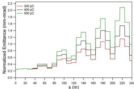
Figure 6: Transverse normalized emittance along aperiodically tuned arc at three bunch charges (initial bunch length 3 psec rms). Breakdown of emittance compensation is evident.
