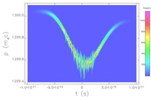
Figure 7: Longitudinal phase after transport of 500 pC through aperiodic arc. Onset of  $\mu$ BI is evident.
