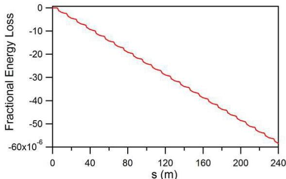
Figure 4: Central energy offset as a function of position through arc, showing uniform loss to CSR emission.
