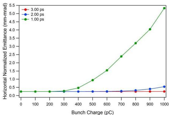
Figure 3: Final transverse emittance as a function of charge for at three initial bunch lengths.
