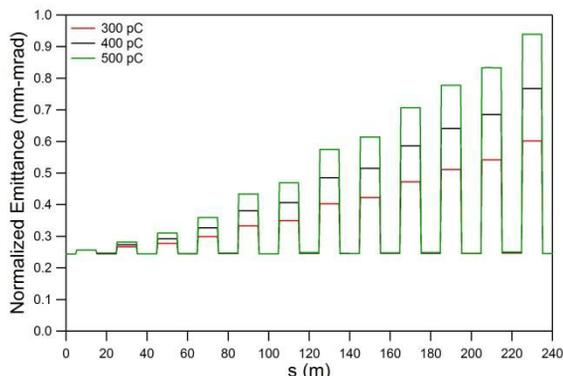
Figure 2: Transverse normalized emittance along the arc at three bunch charges (initial bunch length 3 psec rms).
