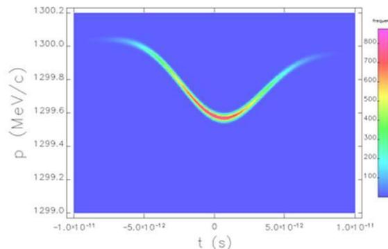
Figure 5: Final longitudinal phase space at 500 pC for initial bunch length of 3 psec rms.
