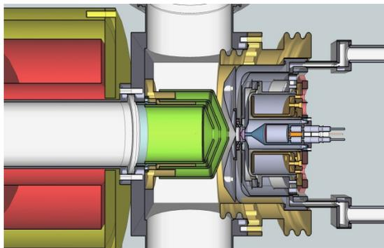
Figure 5: The Duoplasmatron source is on the right. The extraction electrodes are in the center and the 1<sup>st</sup> LEBT solenoid is on the left. Pumps are above and below the electrodes.
