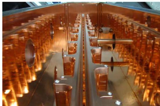
Figure 4: Interior view of the RFQ. The tuning plunger can be seen in the upper-right quadrant of the picture.
