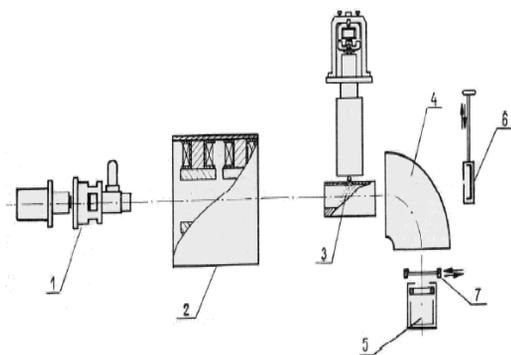
Figure 1: 1 - arc-discharge  $\text{He}^+$  ion source, 2 - quadrupole lens, 3 - sodium jet charge-exchange target, 4 - magnetic analyzer, 5 - Faraday cup with suppressor, 6 - beam profile monitor, 7 - beam profile monitor (scintillator).
