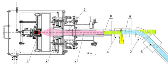
Figure 3: Schematic of an experiment on  $\text{He}^-$  beam production: 1-  $\text{He}^+$  source, 2 - extraction system, 3 - space charge compensation, 4 - Cs (Rb, K) jet target, 5 - bending magnet, 6 - decay channel with solenoid and RF transition, 7 -  $e^+$  beam, 8 - space-charge compensated beam, 9 -  $\text{He}^-$  beam.
