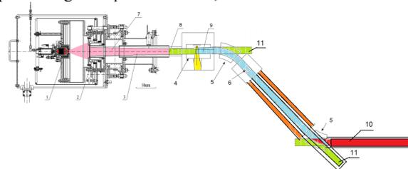
Figure 4: Schematic of a  $^3\text{He}^-$  ion source: 1 - arc-discharge  $\text{He}^+$  source, 2 - extraction system, 3 - space charge compensation, 4 - Cs (Rb, K) target, 5 - bending magnet, 6 - decay channel with solenoid and RF transition, 7 -  $\text{He}^+$  beam, 8 - space-charge compensated beam, 9 -  $\text{He}^-$  beam, 10 - polarized  $^3\text{He}^-$  beam, 11 -  $^3\text{He}$  neutral beam.
