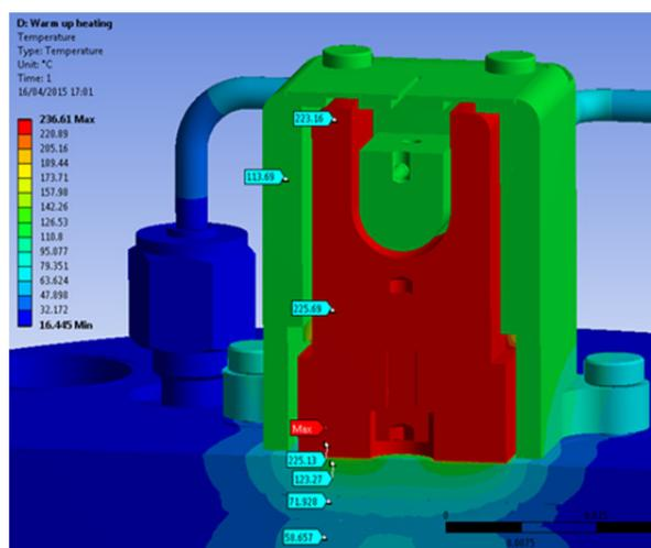
Figure 8: Simulated heating from the cathode heater.
