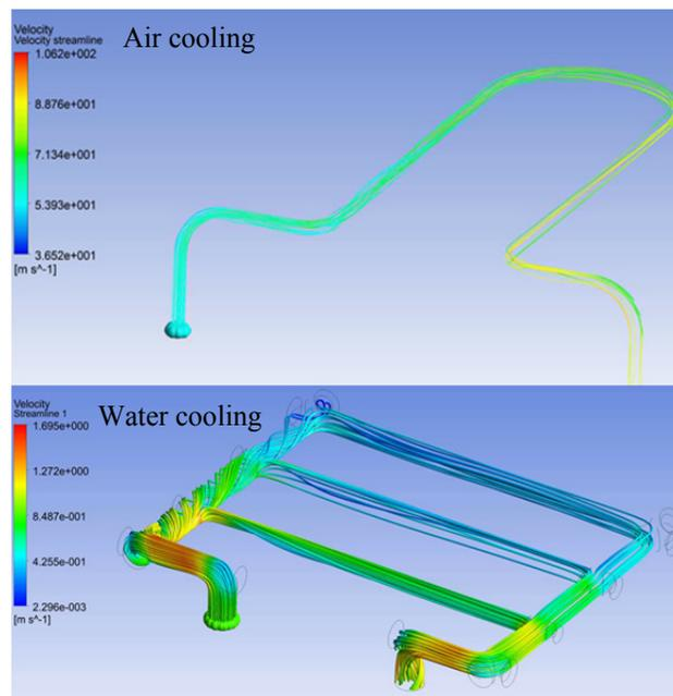
Figure 5: Air and water velocities in cooling channels calculated by CFD.
