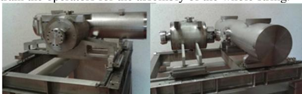
Figure 7: Dummy HWR cavity, solenoid and coupler.
