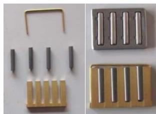
Figure 4: Needle bearing specially developed in order to avoid any magnetization issue. Picture on the left and bottom right show "homemade" bearings with ceramic needle and brass cage. The top right image shows the off-the-shelf rollers originally intended to be used.
