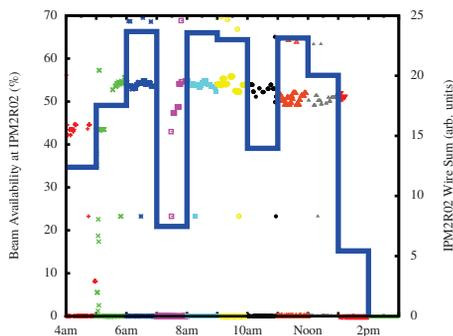
Figure 4: Beam presence in Arc2 as measured by signal on a BPM for eight hours on 2014-02-05. The linacs were set to deliver 1100 MeV/linac, the design energy, during this period.
