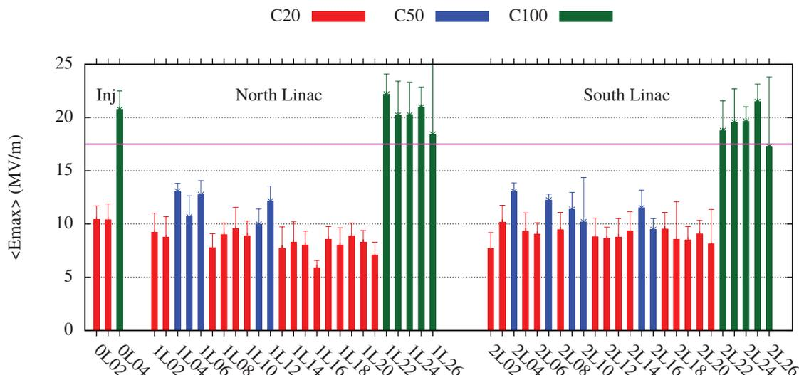
Figure 2: Average maximum cavity gradient per cryomodule as measured prior to the start of 12GeV beam commissioning. The distinction between the C20, C50 and C100 cryomodules is found in the text. The pink line represents the required gradient, 17.5MV/m, needed from the C100 modules.
