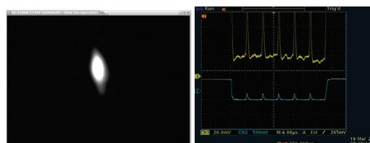
Figure 6: The Arc10 SLM image (left) and the North linac pathlength scope image (right) showing the presence of six beams in the North linac.
