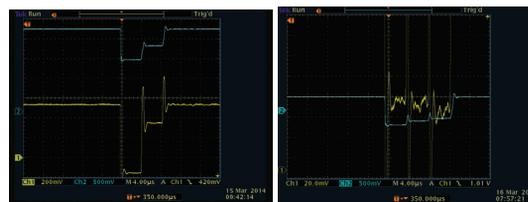
Figure 5: The yellow scope traces represent the relative phase of the different passes in the North linac. The left scope image displays a large difference in phase of about 40° between 1<sup>st</sup> and 2<sup>nd</sup> pass. This was corrected in the right figure (note the different scales, 200 mV/div left, 20 mV/div right) which shows the relative time of arrival of 3-pass beam after a 22 kHz adjustment of the MO frequency.
