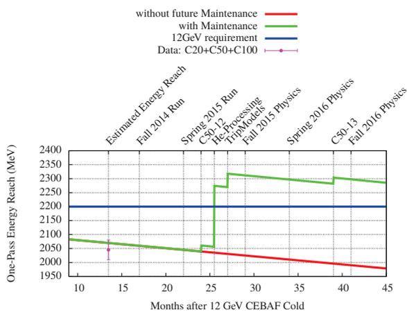
Figure 8: The CEBAF energy reach with and without gradient maintenance. The original CEBAF cryomodule have a measured degradation of about 34 MeV/year.
