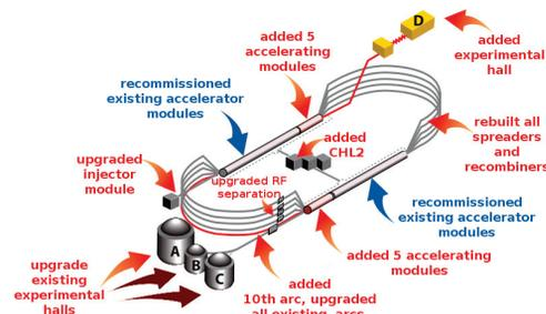
Figure 1: High level overview of the 12GeV upgrade
