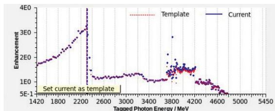
Figure 7: Coherent bremsstrahlung spectrum produced by a 6.6 GeV  $e^-$  beam incident on a diamond radiator.
