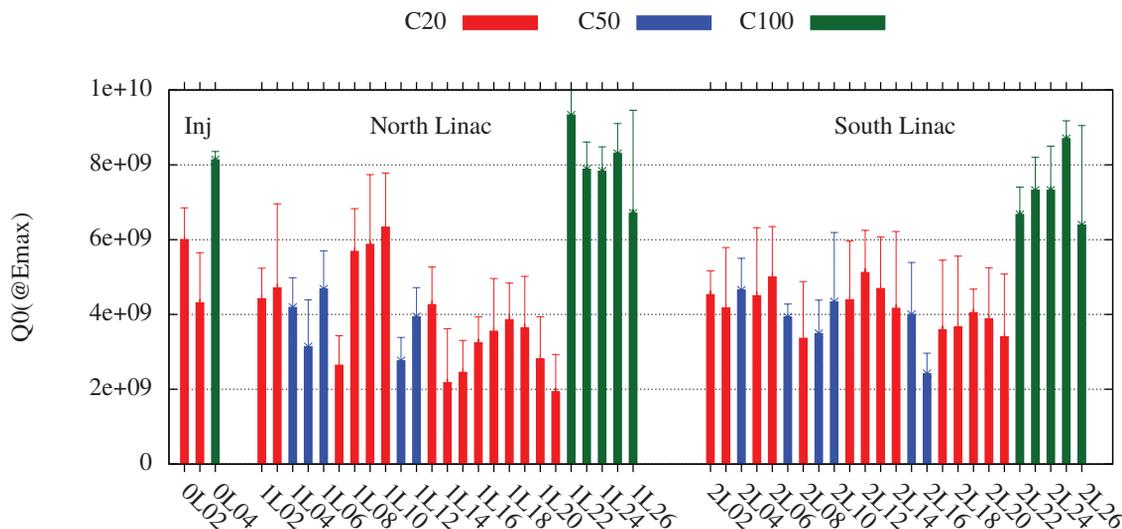
Figure 3: Average cavity  $Q_0$  per cryomodule as measured prior to the start of 12GeV beam commissioning. The distinction between the C20, C50 and C100 cryomodules is found in the text.
