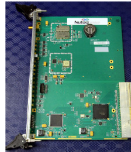
(c) Clock distribution board.
