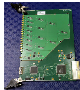
(e) Calibration signal distribution board.
