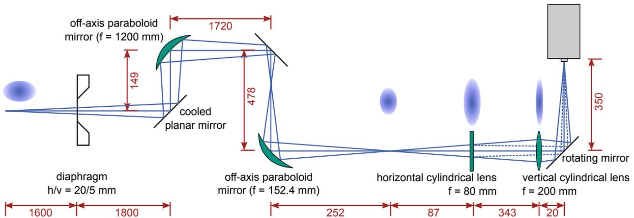
Figure 1: Optical setup for the fast horizontal beam profile measurements. The source point is imaged twice using off-axis paraboloid mirrors of different focal lengths. After the second image the beam ellipse is stretched by cylindrical lenses in order to yield a better resolution on the horizontal plane. For reasons of clarity the dichroic mirrors, used for splitting the light for different experiments, are not included.
