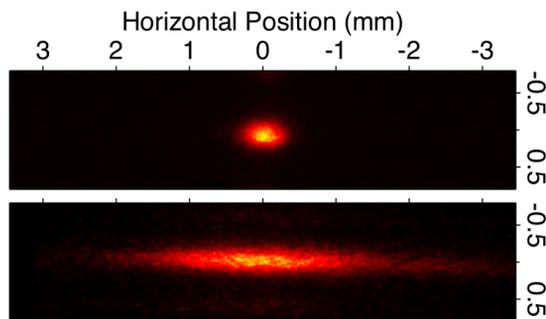
Figure 2: The top figure shows the real image after the second off-axis paraboloid mirror. The beam ellipse is stretched using two cylindrical lenses of different focal lengths, yielding a magnification of 2.6 in the horizontal plane. The stretched image is shown in the lower figure. The images were taken by the fast gated intensified camera and are rotated by 90°.
