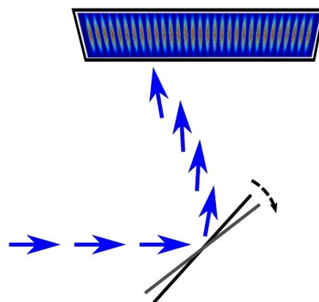
Figure 3: A galvanometric mirror sweeps the transversally stretched synchrotron light pulses over the camera sensor, allowing the observation of horizontal bunch profile fluctuations on short timescales. The camera's fast optical gating ensures the monitoring of a selected bunch, while all other bunches are blanked out.
