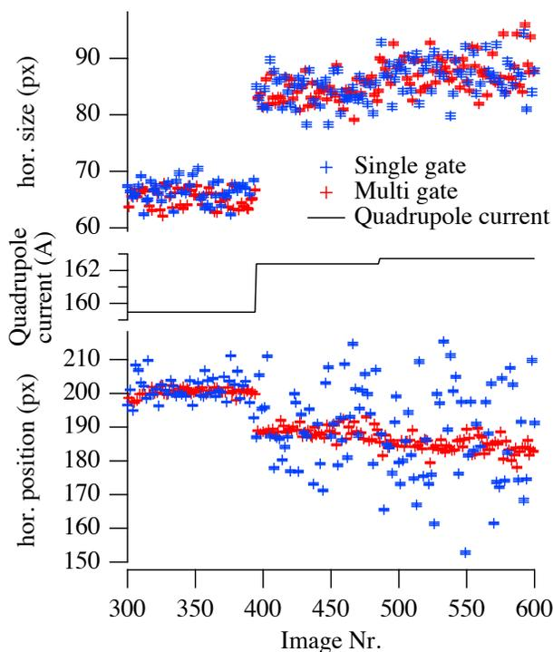
Figure 4: Horizontal spot size and position for single synchrotron radiation pulses (blue) and overlays of about 100 pulses (red) for changing machine parameters. The increase of quadrupole currents causes a reduction of  $\alpha_c$  and hence a decrease of the bunch length. Both the spot size and the position fluctuations of single synchrotron radiation pulses increase for lower values of  $\alpha_c$ .
