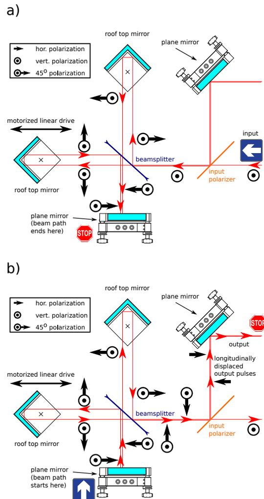
Figure 6: Schematic of the beam path in the two-pass polarizing Fourier-transform spectrometer. The beam polarization is shown for the a) forward and the b) backward pass through the spectrometer.
