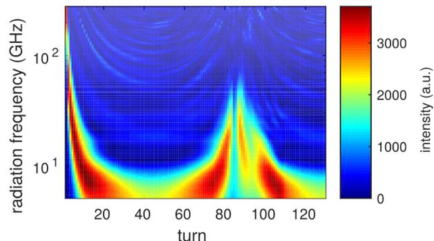
Figure 3: Simulated evolution of the Fourier-transformed longitudinal electron density distribution as function of the number of revolutions.
