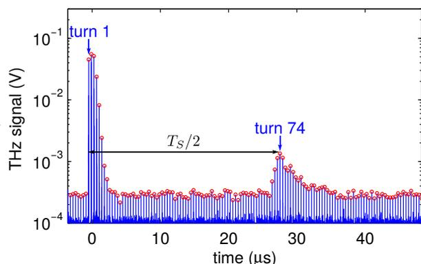
Figure 2: Observation of two pulse trains of laser-induced THz radiation with a time delay matching half a synchrotron oscillation period  $T_S$ .
