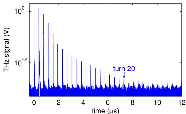
Figure 1: Multi-turn signals from the YBCO detector following a single laser-electron interaction at  $t = 0$  acquired with a 63-GHz oscilloscope showing coherent signals for 20 revolutions.
