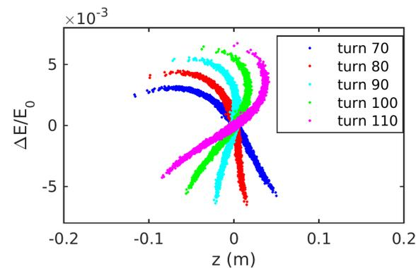
Figure 4: Distribution of energy-modulated electrons in the longitudinal phase space several revolutions after the laser electron interaction.
