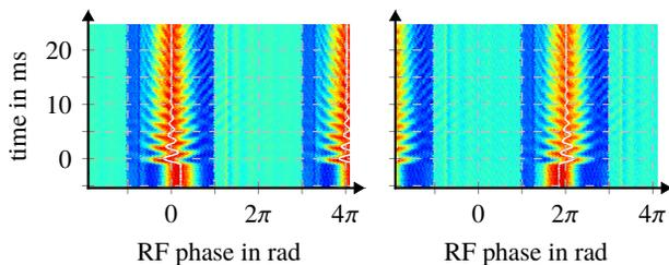
Figure 3: Waterfall plot of single bunches at  $h=2$  with bunch-by-bunch phase detection  $\Delta\varphi$  (white lines) using one DSP system per bunch for an out-of-phase excitation.
