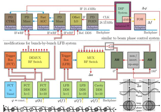
Figure 1: Sketch of LLRF of beam phase control system (top) with modifications for the LFB system (center) and principles of operation (bottom).<sup>1</sup>
