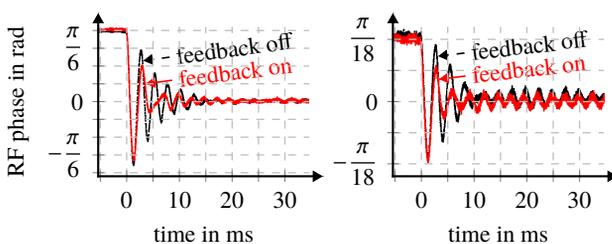
Figure 5: Comparison of open and closed loop operation.
