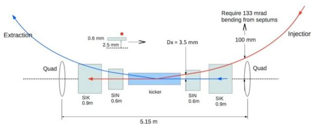
Figure 1: Layout of the ALS-U lattice in the injection/extraction straight.
