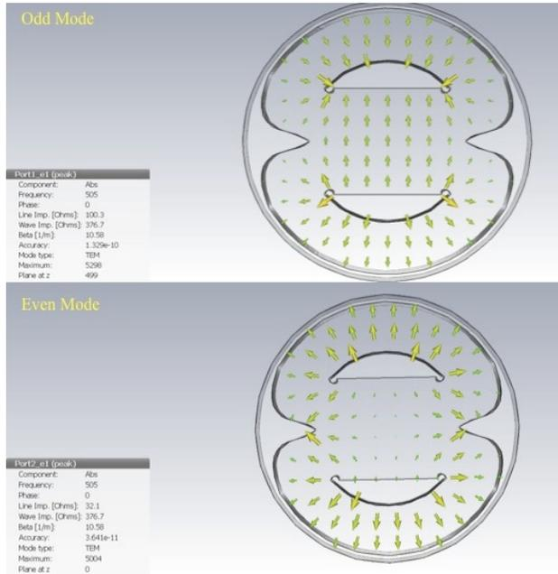
Figure 3: Transverse section of stripline kicker with electric field map for differential (top) and common mode (bottom). Characteristic impedances are  $Z_{\text{odd}} = 50 \Omega$  and  $Z_{\text{even}} = 64 \Omega$ .
