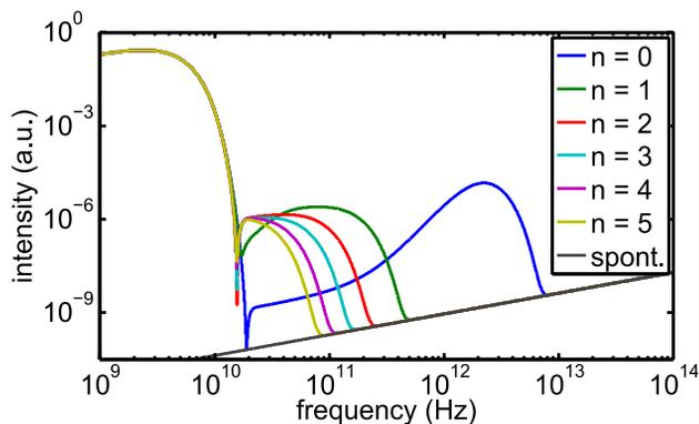
Figure 6: Simulation of the THz spectrum for revolutions  $n = 0$  to 5 after an initial laser-electron interaction. For reference, the spontaneous incoherent bending magnet spectrum is also shown.
