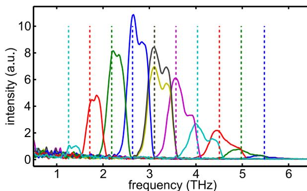
Figure 8: Coherent narrow-band THz spectra, normalized to the bunch current and recorded using different settings of the Michelson interferometer. The modulation frequencies of the laser pulse, measured by an optical autocorrelator, are shown as dashed lines.
