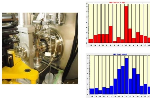
Figure 6: (Left) Si PIN diodes located around beam pipes and (right) example of radiation data taken by those Si PIN diodes.
