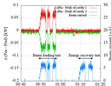
Figure 5: Energy recovery trial. Beam loading effect cannot be seen on “Energy recovery test”. In the Beam loading test, upper and lower cavity only accelerates and decelerates electron beams.
