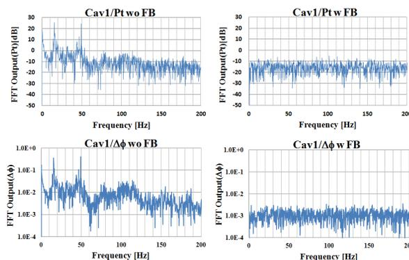
Figure 1: Microphonics of LLRF.
