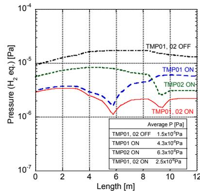
Figure 4: Pressure distribution which is calculated by the code VASCO. The dotted and solid line represents the pressure ( $\text{H}_2$  eq.) without and with the additional pumps.
