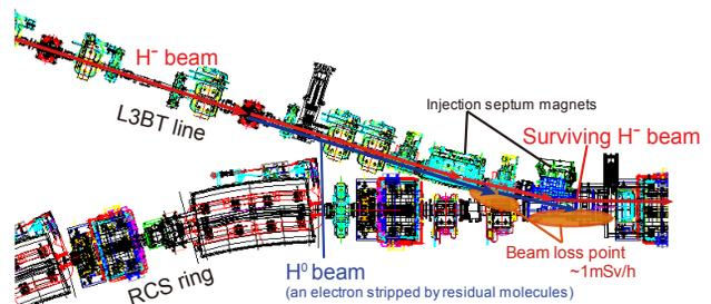
Figure 1: Layout of L3BT line near the injection section of RCS. The possible mechanism of the beam loss is also shown.
