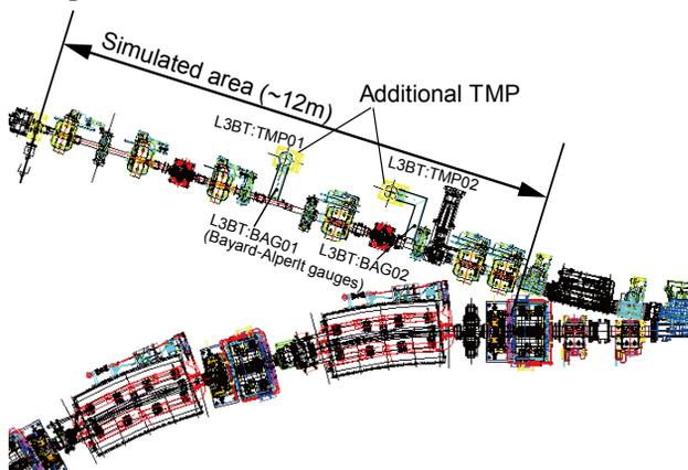
Figure 3: Arrangement of turbo molecular pumps in L3BT line. The area, which was simulated by the calculation code, was also shown.
