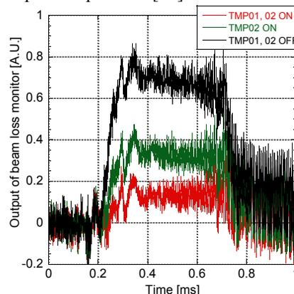
Figure 6: Measured beam loss signal in each case with and without additional TMP.
