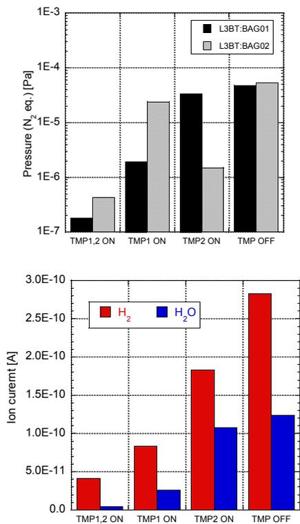
Figure 5: Measured beam line pressure in each case with and without additional TMP.
