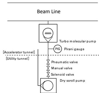
Figure 2: Schematic block diagram a turbo molecular pump unit.
