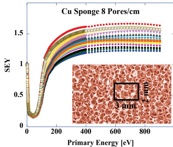
Figure 1: SEY spectra obtained by moving the  $e^-$  beam in small steps in a  $2 \times 3$  mm<sup>2</sup> area within a 8 pores/cm Cu foam mounted in a  $6 \times 6 \times 6$  mm<sup>3</sup> Cu cage, and their mean value. The inset shows the picture of the 8 pores/cm Cu foam, and the geometrical region (black rectangle) where the SEY curves have been measured.
