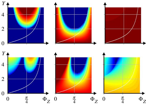
Figure 3: Damping, coherent dipole and quadrupole frequency (left to right) for short (top) and long (bottom) bunches; with color bar from  $\omega_{\text{syn},0}$  to  $2\omega_{\text{syn},0}$  for the quadrupole frequency and from 0 to  $\omega_{\text{syn},0}$  otherwise.
