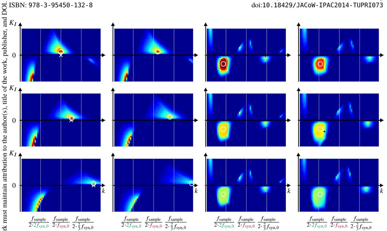
Figure 4: Impact of (relative) beam loading,  $Y \in \{0, 0.75, 1.5\}$  (top to bottom), on the closed loop performance for damping of dipole (left) and quadrupole (right) oscillations for short and long bunches, respectively.
