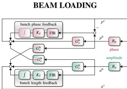
Figure 1: Block diagram for small modulation with the notation of [3] ( $p$ : phase,  $a$ : amplitude,  $v$ : voltage,  $b$ : beam and  $G_s^b$ ,  $G_c^b$ ,  $B_p$ ,  $B_a$ : transfer functions, see also Eqs. (1-5)).
