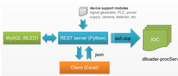
Figure 4: Overview of DCDB architecture.
