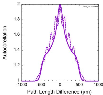
Figure 4: Calculated autocorellation traces for the un-modulated bunch profile of Fig. 2 (continuous line) and for the calculated model profile of Fig. 3 (dashed line).
