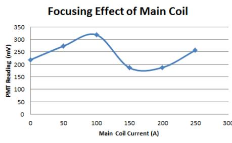
Figure 4: Scan of Main Coil Field Strength.
