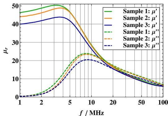
Figure 4: Complex relative permeability spectra of three samples with different bias history.
