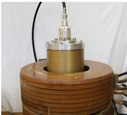
Figure 3: Measurement set-up: Sample holder in solenoid.
