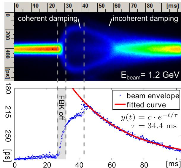
Figure 5: Coherent and incoherent damping observed when the bunch-by-bunch feedback was switched off for 5 ms.
