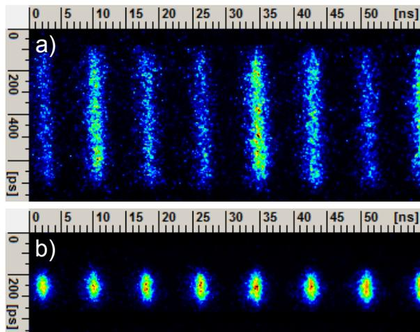
Figure 4: Comparison of synchroscan measurements: Single shot image of strong incoherent longitudinal particle oscillations around the reference phase at 1.2 GeV and 145 mA beam current (a) and damped bunches at standard beam current (b).
