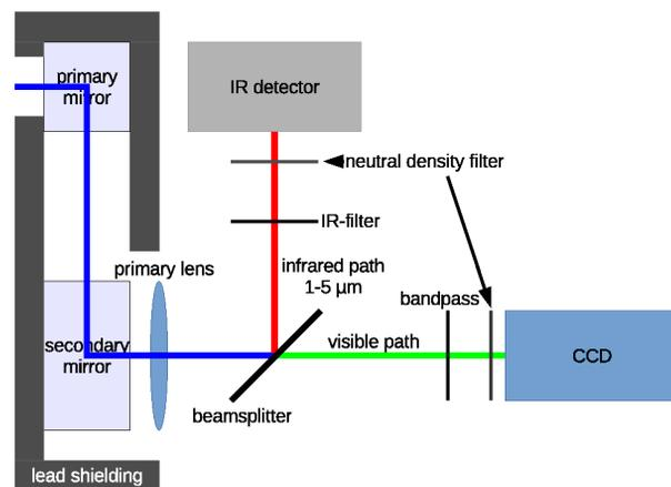
Figure 4: Scheme of the two planned optical paths.
