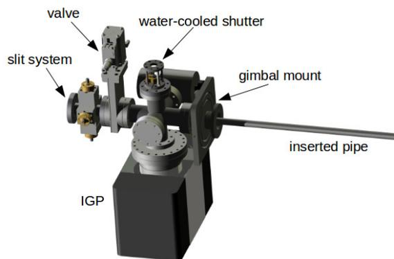
Figure 2: Set-up of the front end components.
