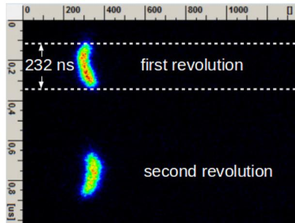
Figure 6: Streak camera image of the circulating bunch train in the pulse stretcher ring after the first injection. Horizontal oscillation is shown while the bunch train passes by two times. Each bunch train being 232 ns long.
