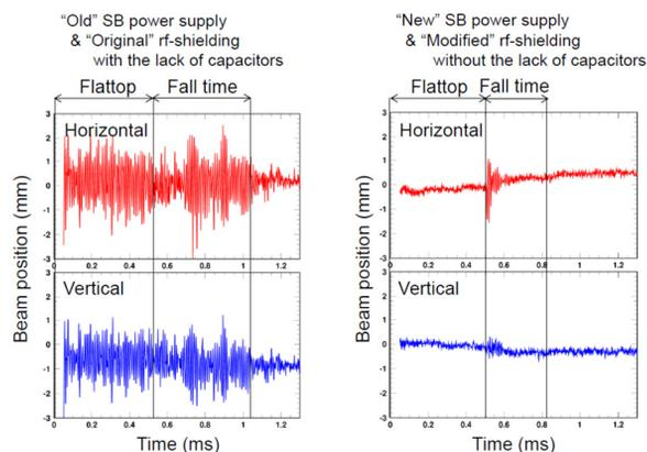
Figure 1: Beam position moving due to SB induced dipole ripple both previous and new power supply.
