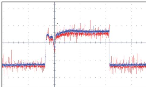
Figure 7: Beam signals from ACCTs before (blue) and after (red) RFQ.
