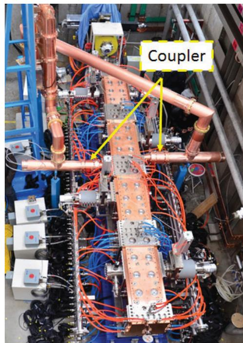
Figure 4: The injector II RFQ on site.
