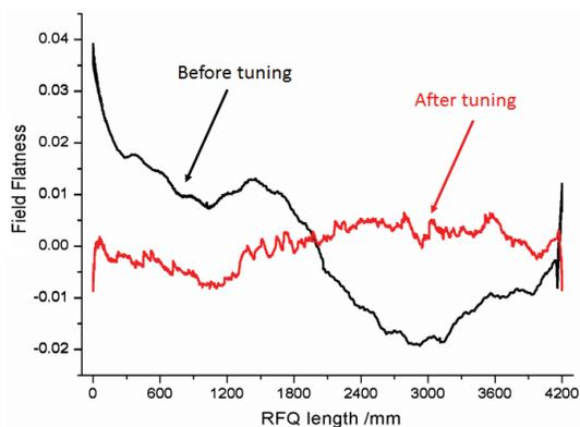
Figure 3: Field flatness before and after tuning.
