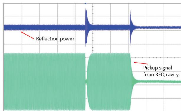
Figure 5: Sparking signal in cavity and transmission line.
