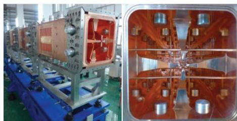
Figure 1: External and internal view of injector II RFQ.
