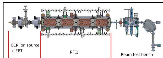
Figure 6: The injector II RFQ acceleration system.
