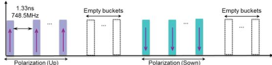
Figure 3: Bunch train and polarization pattern in the MEIC electron collider ring.
