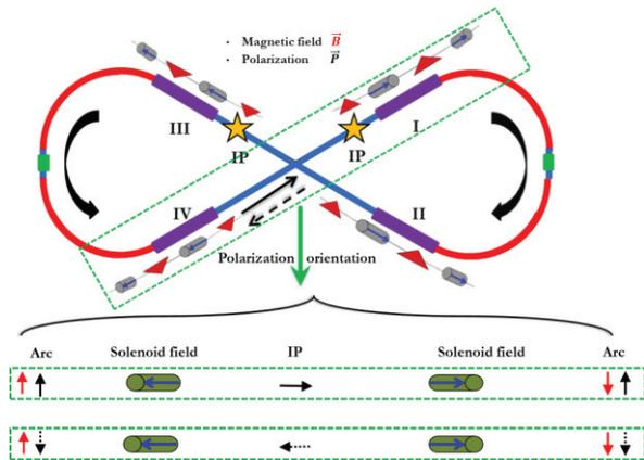
Figure 2: Polarization ( $\vec{P}$ , black arrow) directions remain same in the two arcs by having opposite longitudinal solenoid field directions in the same long straight. The blue arrow in the solenoid represents the field direction. The polarization orientation in one of the two long straights (shown in the green box) is exhibited under the half brace with two different polarization states at the IP.
