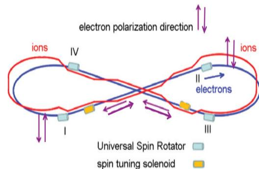
Figure 1: Polarization configuration in the MEIC electron collider ring.
