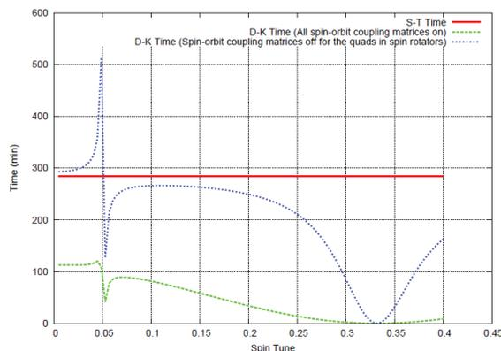
Figure 5: Example of spin tune scan at 5GeV MEIC electron collider ring.
