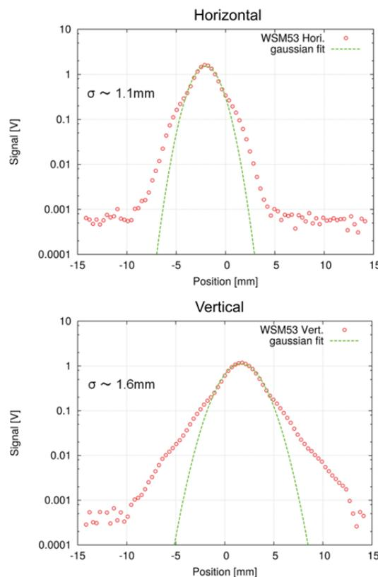
Figure 3: Transverse beam profile at the WSM in the L3BT scraper section. The red dots are the measurement results by the WSM and green lines are gaussian fitting results.
