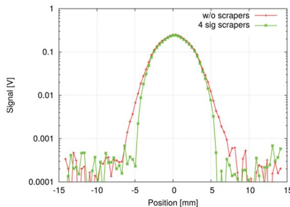
Figure 4: Scraped beam profile in the vertical direction. Red lines are vertical beam profile without setting scrapers, green lines are beam profile with setting scrapers.
