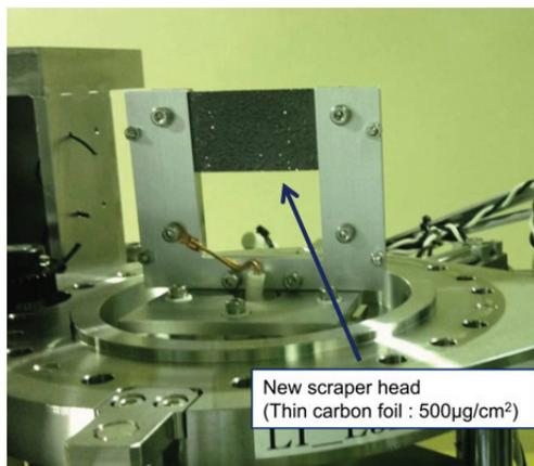
Figure 2: Picture of the new scraper head with the thin carbon foil. The carbon foil is mounted by the metal foil folder.
