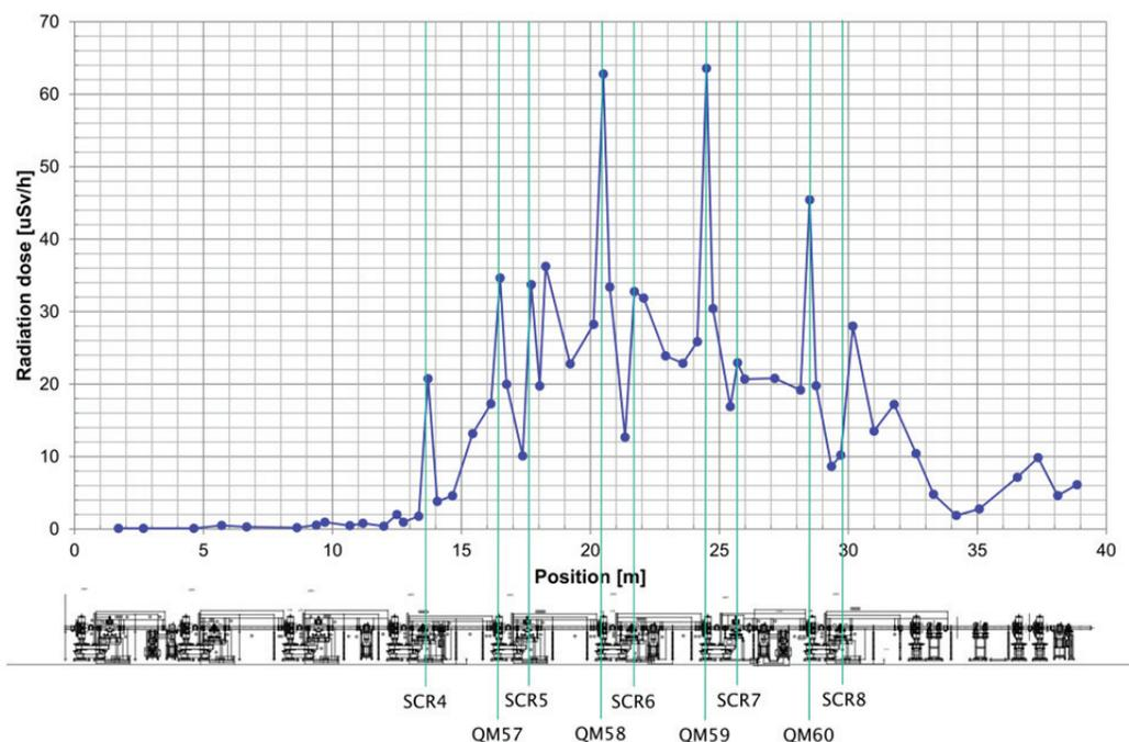
Figure 5: Figure of the radiation dose around the scraper section after 2 days user operation. Localized radio-activation was observed at the new scrapers and the quadrupole magnets.
