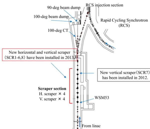
Figure 1: Schematic layout of the L3BT scraper section and the 100-deg dump.
