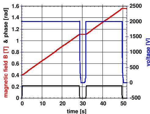
Figure 4: Magnetic field ramp (red) to accelerate the uranium beam from  $740 MeV/u$  to  $4.5 GeV/u$ . The intermediate flat top at  $3 GeV/u$  has a duration of  $3 s$ . During acceleration the cavity voltage is constant  $2 kV$ .
