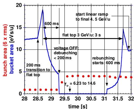
Figure 7: Bunch area (6 times rms, red) and bucket area (blue) in the intermediate flat top region. Transition gamma is changed from  $6.23$  to  $14.6$  when the beam is completely debunched ( $29.7$  s).
