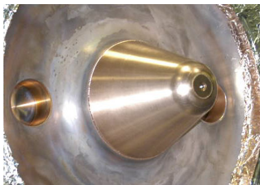
Figure 4: Cathode assembly after Ebeam welding.
