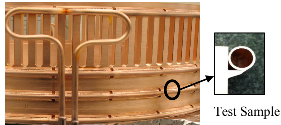
Figure 5: Fusion weld of cooling tube to cavity wall.
