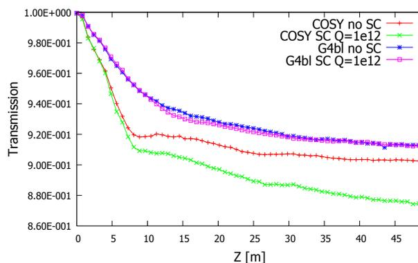
Figure 5: Plot of transmission rate through 60 cells of late stage muon cooling channel, with and without space charge. The difference in transmission is due to issues with longitudinal dynamics, as well as a larger space charge effect in COSY.
