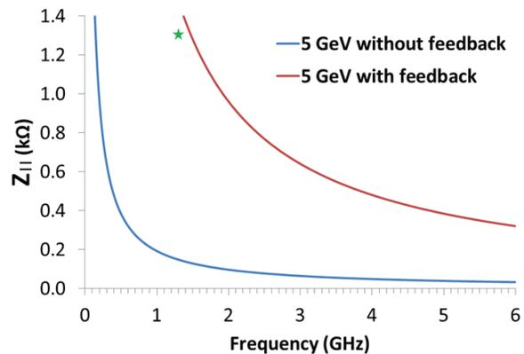
Figure 2: The longitudinal impedance threshold with and without feedback system for electron ring cavities. The green star indicates the impedance of the  $TM_{011}$  mode.
