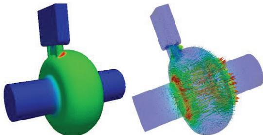
Figure 3: SRF cavity concept with one on-cell damper, TM<sub>010</sub>. Left, surface magnetic field, right, electric field.
