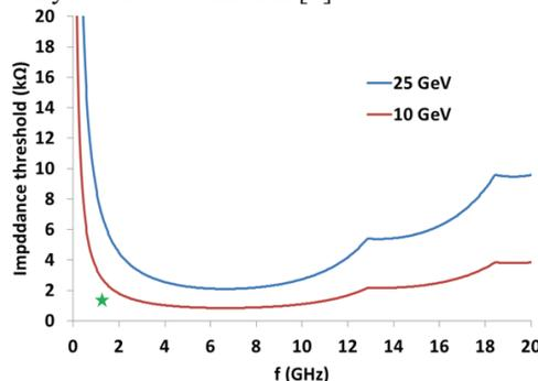
Figure 4: Impedance threshold for ion ring, the green star indicates the cavity's impedance is below threshold.
