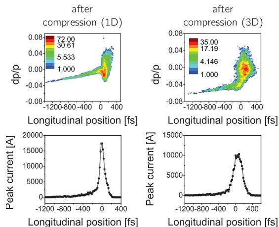
Figure 5: Longitudinal phase space distributions and bunch profiles for a bunch charge of 3 nC after compression. The transverse beam size is increased by a factor of 5 compared to Fig. 2. The difference between the 1D and 3D simulations is significantly smaller.
