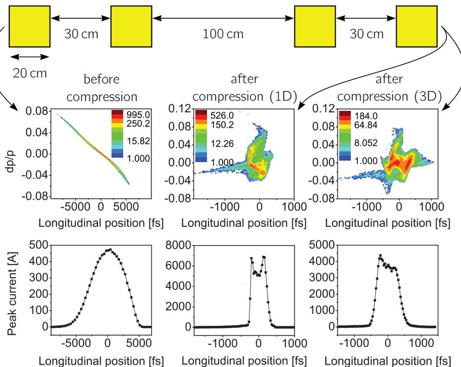
Figure 2: Longitudinal phase space distributions and bunch profiles for a bunch charge of 3 nC before and after compression using 1D ( $L_{\text{rms}} = 199$  fs) and 3D simulations ( $L_{\text{rms}} = 270$  fs).
