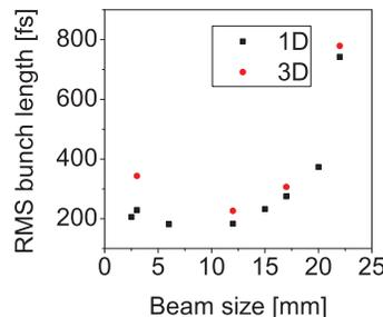
Figure 6: Compressed bunch length as a function of transverse beam size for a bunch charge of 3 nC and an energy of 40.8 MeV. For reasons of demonstration the space charge density was artificially decreased by expanding the transverse beam size far beyond the design values. Results for 1D and 3D options converge at lower charge densities, i.e. bigger beam sizes.
