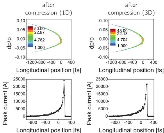
Figure 4: Longitudinal phase space distributions and bunch profiles for a bunch charge of 3 nC after compression. The bunch energy is increased from 40 MeV (Fig. 2) to hypothetical 300 MeV with the dipole field adjusted accordingly.
