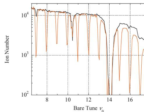
Figure 4: Experimental excitation of integer stopbands (red) using the dipole perturbation (black) without dipole perturbation.
