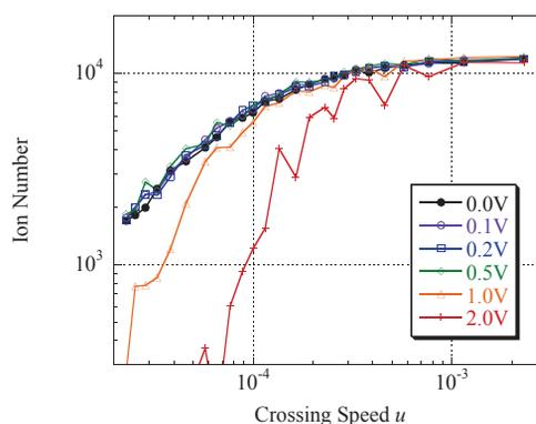
Figure 7: Multiple resonance crossing of the whole EMMA tune range for varied dipole amplitude at various crossing speeds.
