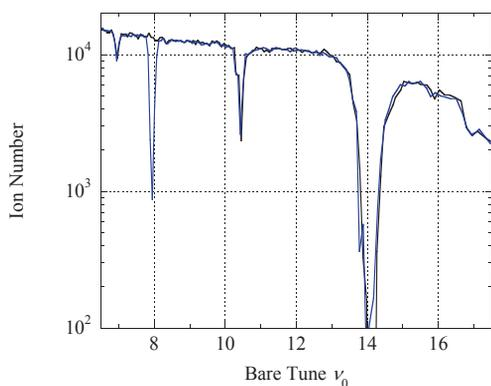
Figure 5: Excitation of the dipole stopband at one integer (blue) with control over fourier harmonics. The spectrum without dipole perturbation is shown in black.
