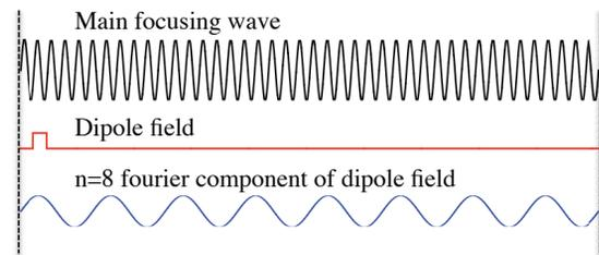
Figure 3: Schematic of the dipole pulse perturbation (red) and the  $n=8$  fourier harmonic (blue) of the pulse together with the main focusing waveform (black).
