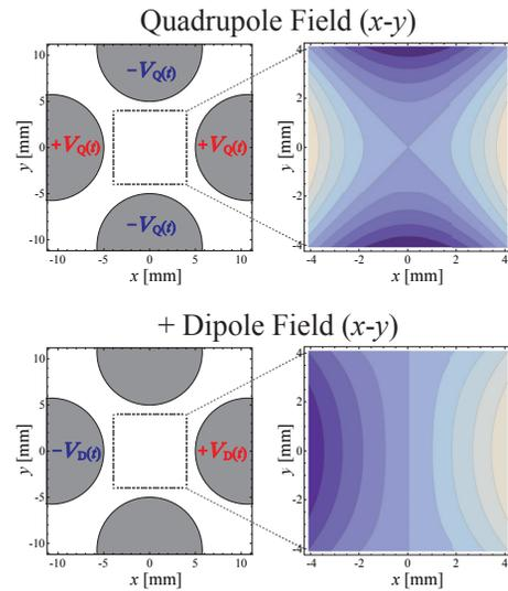
Figure 2: Schematic layout of the S-POD rods and the creation of quadrupole (focusing) and dipole (perturbative) electric fields.
