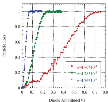
Figure 6: Single resonance crossing of the  $\nu_0 = 12$  integer resonance for varying dipole amplitude at various crossing speeds.
