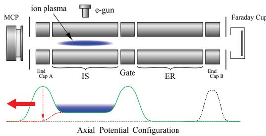
Figure 1: Schematic layout of the linear Paul trap with the confinement potential configuration.
