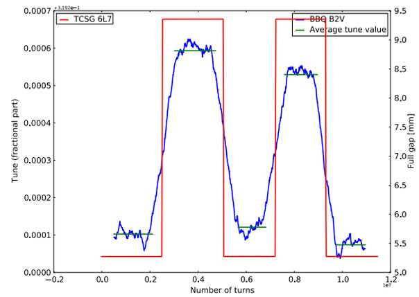
Figure 4: Tune vs. time when the TCSG in IR7 are moving, with transverse damper on, during the MD of June 2012. One of the TCSG gap (twice the half gap, which varies between  $5.1$  and  $9\sigma$ ) is also shown (in mm units).
