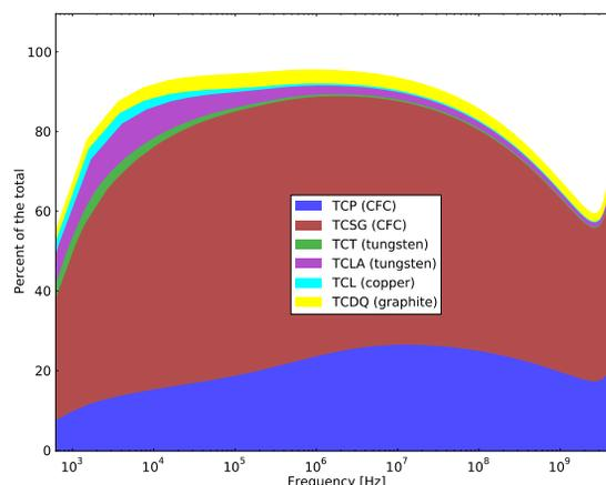
Figure 2: Contributions (in percent) of various collimator families to the total vertical dipolar impedance (imaginary part) at 4 TeV (squeezed optics) with typical 2012 collimator settings [10]. See Fig. 1 for the acronyms definitions.
